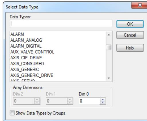
If you want to define the tag as an array, in the **Array Dimensions** boxes, enter the number of elements in each dimension.
