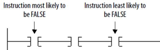
When the controller finds a false instruction, it executes the remaining instructions in the series with their rung-condition-in set to false. Typically, an instruction executes faster when its rung-condition-in (rung) is false rather than true.
