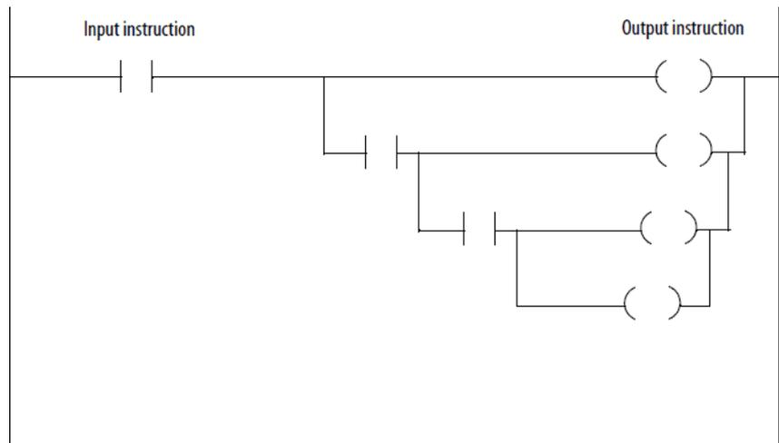
Large rungs with complex, nested branches result in having to scroll through the ladder editor and may end up spanning multiple pages when you print the logic. To make it easier to maintain, divide the logic into multiple smaller rungs.
