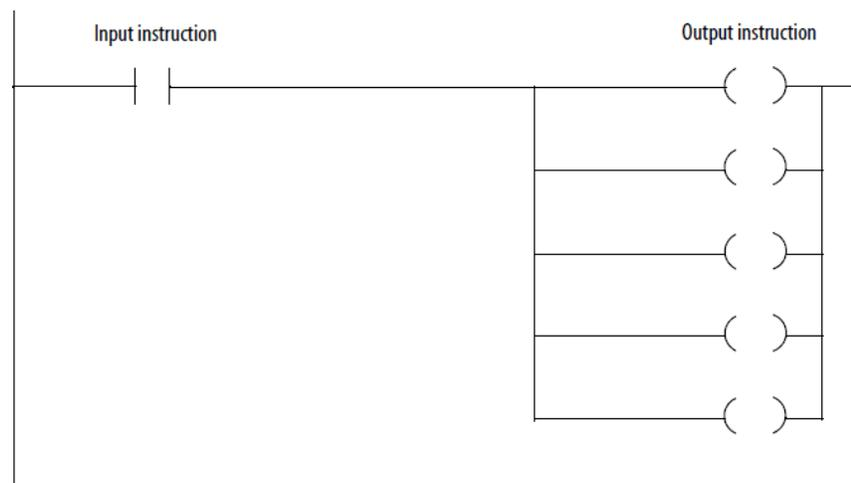
You can nest branches to as many as 6 levels. This example shows a nested branch. The bottom output instruction is on a nested branch that is three levels deep.
