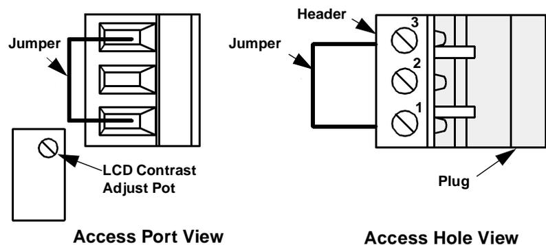
The jumper may be removed and an externally mounted user-supplied key switch connected.
