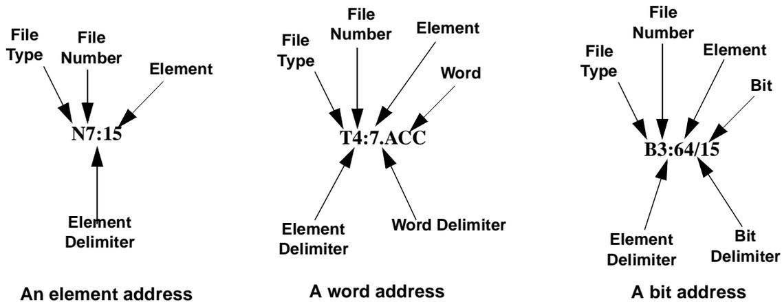
The address format varies, depending on the file type. This is explained in the following sections. We begin with file 0 and 1, outputs and inputs, and follow with files 3, 4, 5, 6, and 7.
