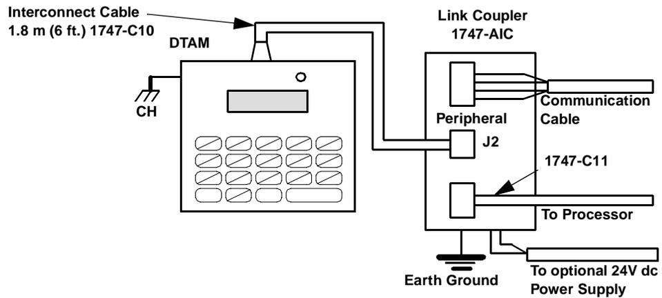
You can connect the DTAM module to an SLC 5/04 or later processor using either of the following methods.
