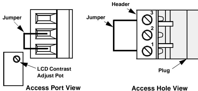
To configure the module for the **Monitor** mode, either connect the jumper between terminals 1 and 3 (leaving the jumper installed in the module) or completely remove the jumper. You may either leave the header in place and make the connection via the access port and access hole, or temporarily remove the header from the module by pulling it off of the plug. If you choose the latter method, return the header to the plug once the connection is made.
