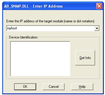
To specify the network path, in the device path box, enter the IP address or host name of the target module. Click **OK** to go to the Firmware Revision dialog box.
