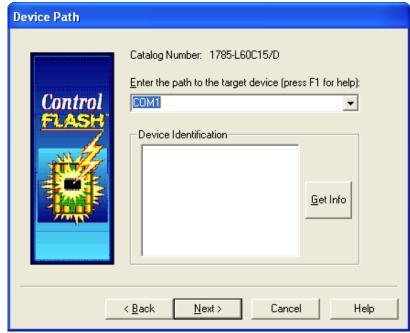
To specify the network path, in the device path box, enter the path in the box of the target module. Click **Next** to go to the **Firmware Revision** dialog box.
