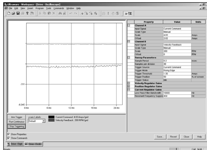
Figure 5.11 shows the effect of the Low Pass Filter. The Low Pass Filter parameter is set to 458 Hz, and the Resonant Frequency Suppression is set to
