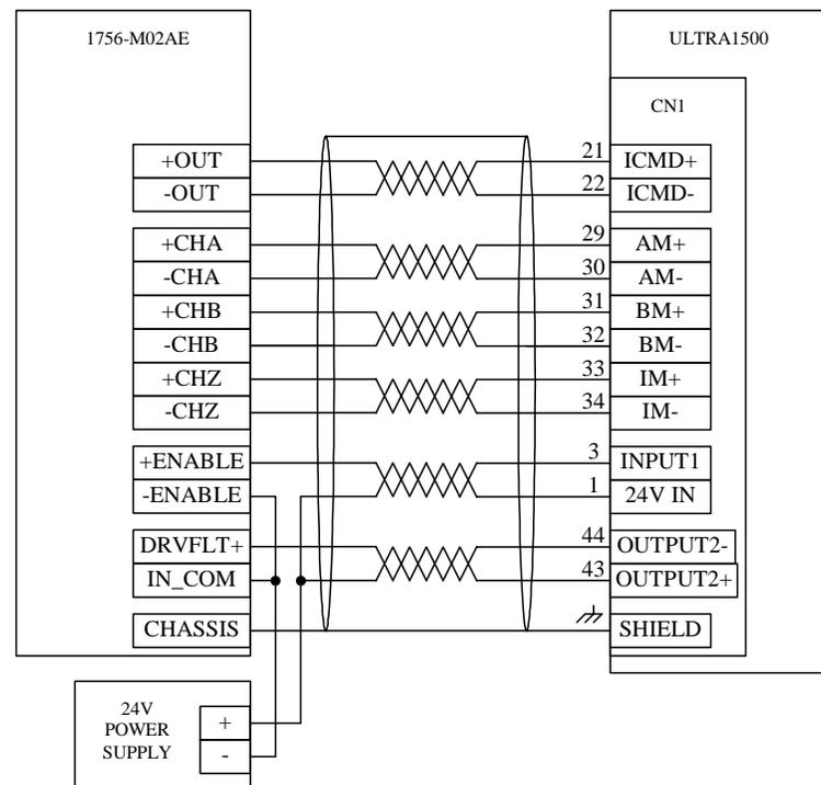
In Figure 5.1, the 1756-M02AE provides a current command to the drive and the 1756-M02AE closes the velocity loop. Alternatively, the 1756-M02AE can provide a velocity command to the drive, and the drive can be responsible for the velocity loop closure. In that case, the 1756-M02AE command outputs should be connected to CN1 pins 19 and 20, instead of CN1 pins 21 and 22, and the Ultra1500 should be operated in Analog Velocity mode.
