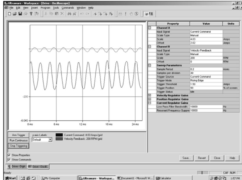
Figure 5.10 shows the effect of the Resonant Frequency Suppression filter. The Resonant Frequency Suppression parameter is set to 458 Hz, the Low Pass Filter is set to 10000 Hz. The current and velocity waveforms appear very smooth as compared to the original waveforms.
