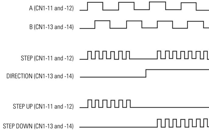
Figure 2.9 shows the configuration of the Position Command inputs, and the following table provides descriptions of these inputs.
