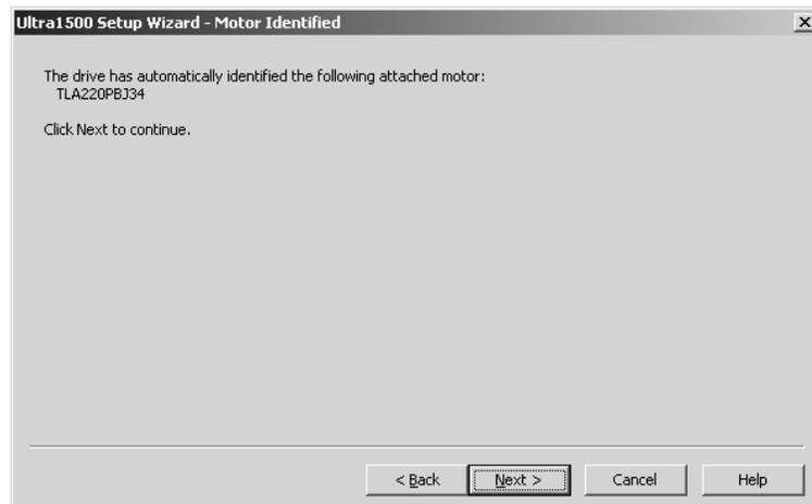
7. After the motor is selected, the Setup Wizard allows an autotune procedure to execute. Autotune sets the tuning gains to values appropriate for the motor and load.
