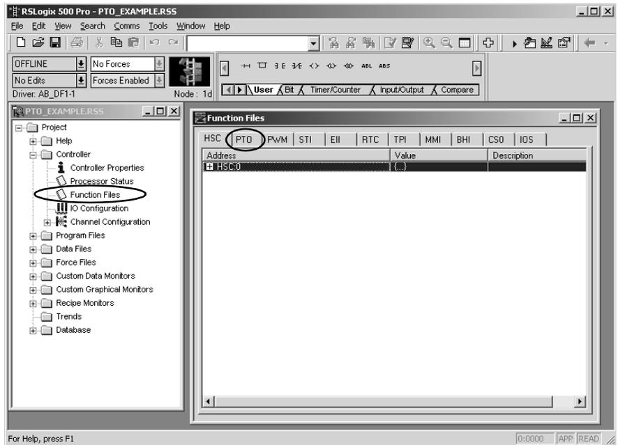
Select the **PTO** tab of the function files window to access all PTO-related configuration parameters:
