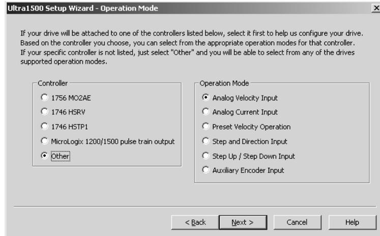
5. Depending on the Controller and Operation Mode selections, the next one or two screens prompt for configuration settings that are applicable.
