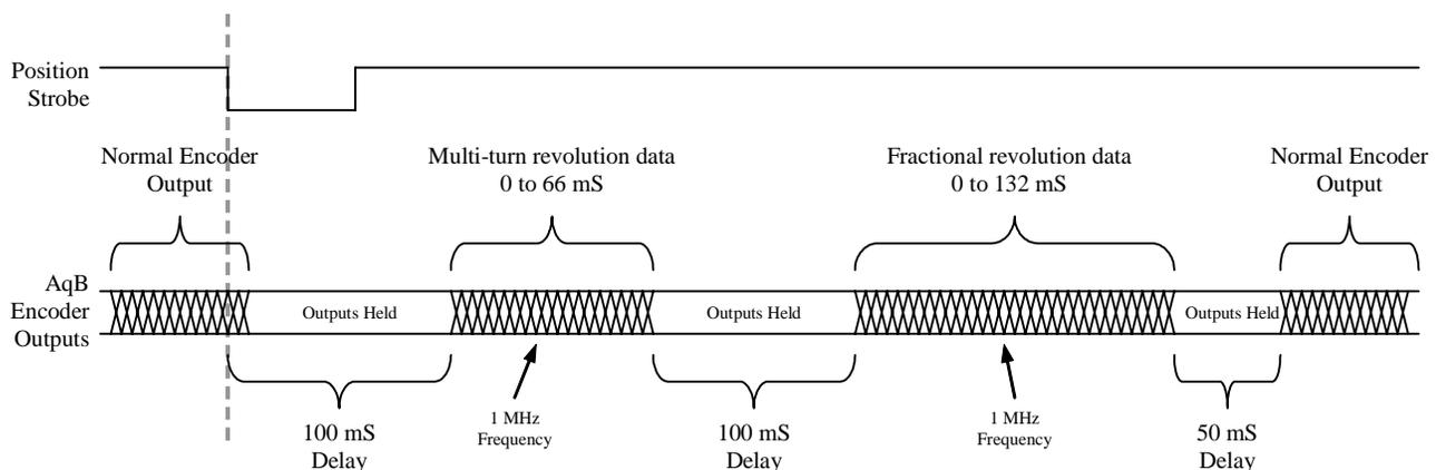
In Figure 5.6 it can be seen that the drive hardware and firmware executes the following sequence when the active-going transition of the Position Strobe input is detected:
