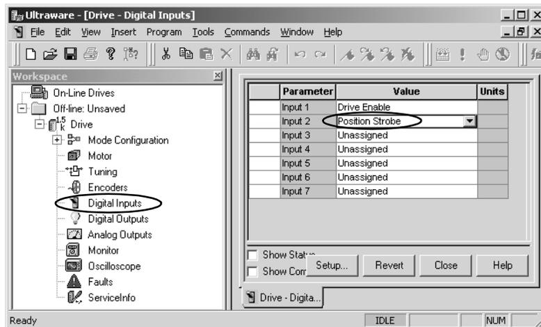
The active-going transition (an active state is when the opto-isolator is turned ON and the input voltage is 0V) of the Position Strobe input starts a time-based sequence in which the absolute position data is transferred via the A and B encoder outputs of the drive, as shown in Figure 5.6.
