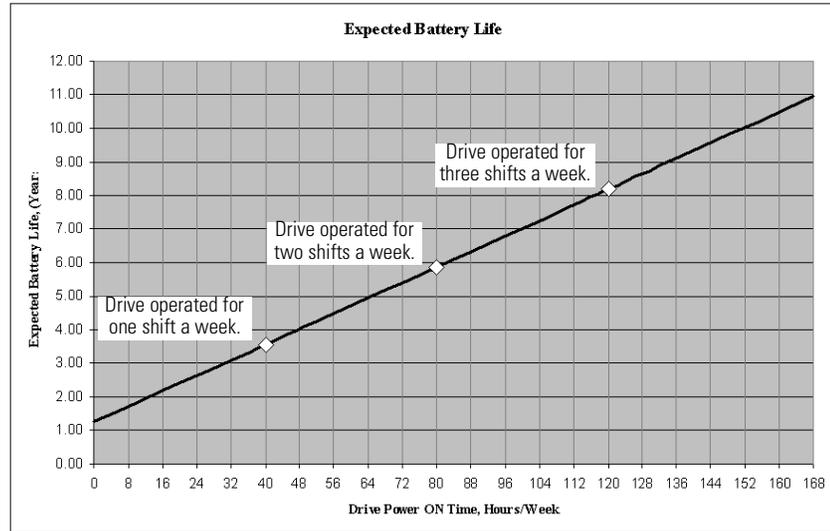
In Figure 5.5, three data points are highlighted. For example, if the control power of the drive is applied for 40 hours per week, (and the encoder uses battery power the remaining 128 hours in the week), the expected battery life is about 3.5 years. In applications where machine downtime is a concern, replacing the battery once a year or once every two years may be a prudent measure to avoid any interruption.
