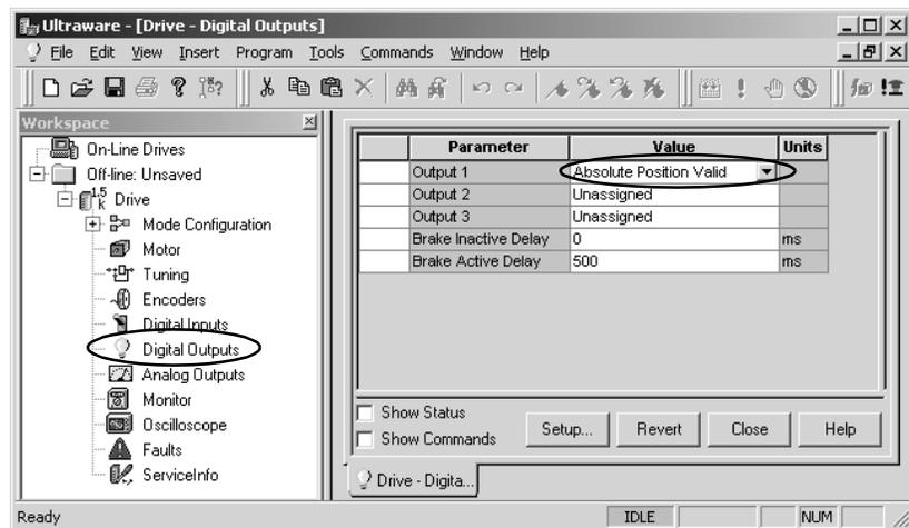
This signal is used by the controller to indicate when absolute position motion is not possible, and a homing procedure is necessary.
