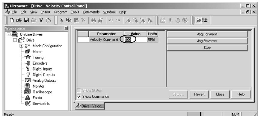
3. Enter an appropriate low speed in the Velocity Command value field.
