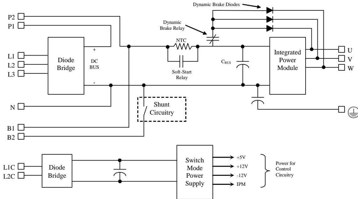
Note: DC Bus Negative is labelled N on the drive cover, but DC- on the removable connector.
