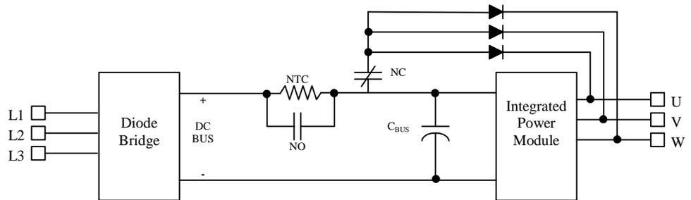
In the figure, it is important to notice that the dynamic brake relay contacts utilize the same controlling coil as the soft-start thermistor circuitry. This interdependence can be important in certain applications. The possible states of the dynamic brake and soft start contacts are as follows:
