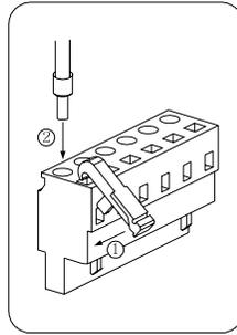
1. Open terminal locking clamp with connector tool as shown.
