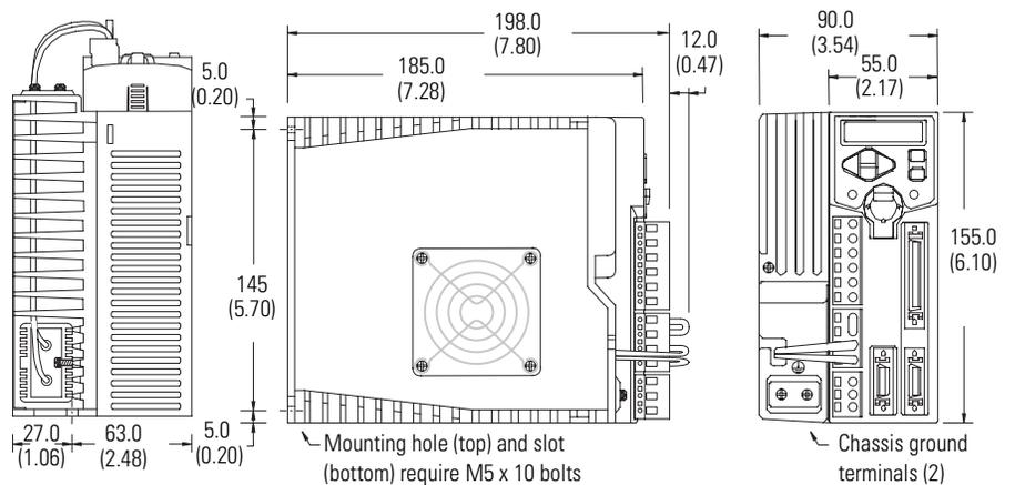
Dimensions are in millimeters (inches). Drives are designed to metric dimensions; inches are a mathematical conversion.
