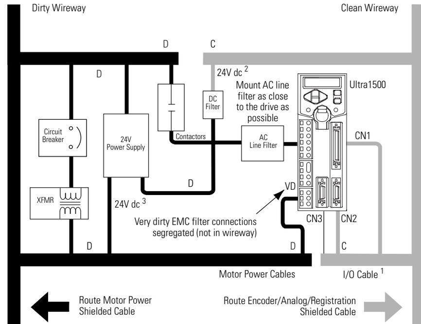
1 If I/O cable contains (dirty) relay wires, route cable with motor (output) power wires in dirty wireway.
