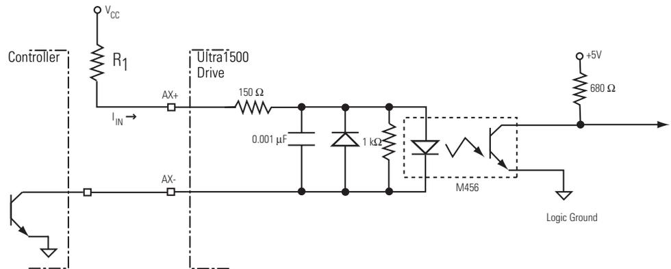
R<sub>1</sub> must be chosen so that the input current, I<sub>IN</sub>, is between 7mA and 15mA for an ON state to be recognized:
