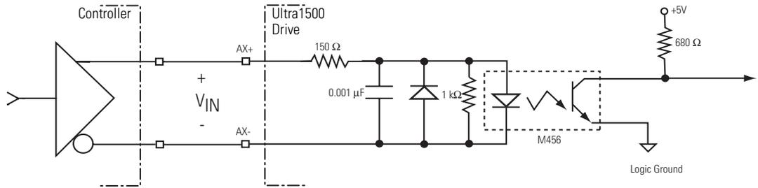
V<sub>IN</sub> must be between 2.8V and 3.7V for an ON state to be recognized.
