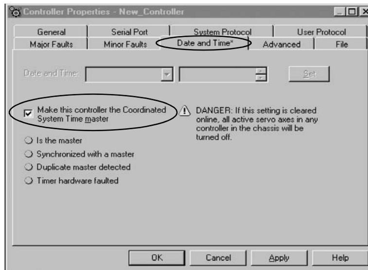
6. Check the box **Make this controller the Coordinated System Time master**.
