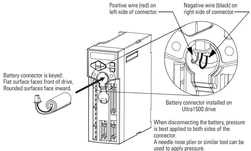
To install a new battery, or replace an existing battery; perform the following steps:
