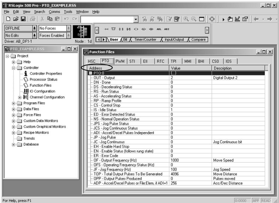
The PTO settings are typically embedded in the program instructions, with some of the settings initialized at the start of the program, and others set according to the application needs.
