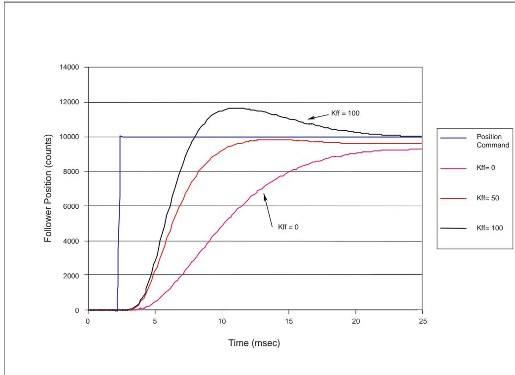
Figure 5.17 illustrates the effect of the  $K_{ff}$  gain on the follower response or position error for a typical motion profile. The steady state error is reduced as the  $K_{ff}$  term is increased. When  $K_{ff}$  is 100, the steady state error is almost zero, but there is some error during the acceleration and deceleration portions of the profile. The velocity loop tuning can determine the effectiveness of the position loop feedforward term.
