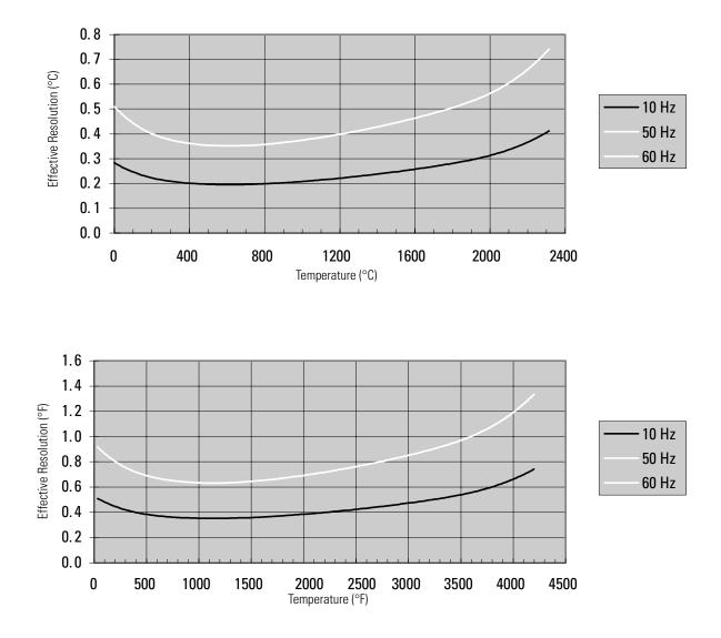
Figure 3.4 Effective Resolution Versus Input Filter Selection for Type C Thermocouples Using 10, 50, and 60 Hz Filters
