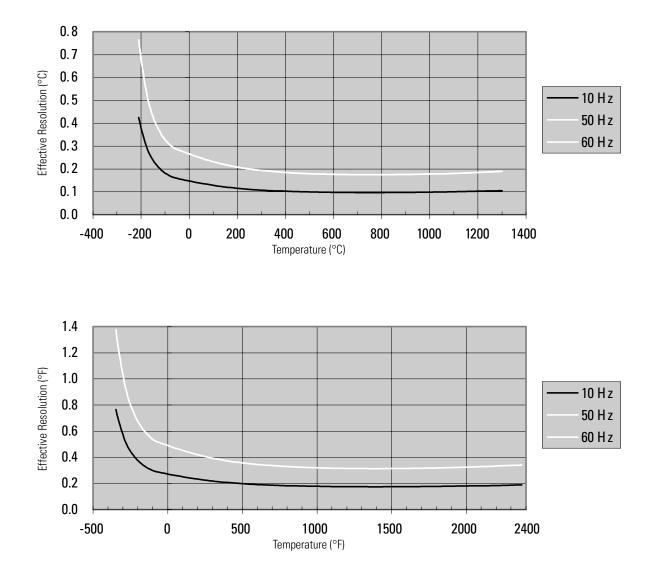
Figure 3.12 Effective Resolution Versus Input Filter Selection for Type N Thermocouples Using 10, 50, and 60 Hz Filters
