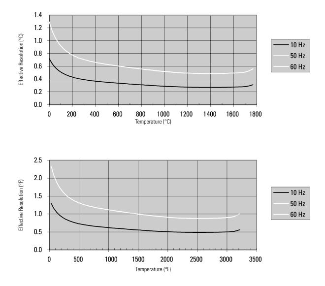
Figure 3.14 Effective Resolution Versus Input Filter Selection for Type R Thermocouples Using 10, 50, and 60 Hz Filters
