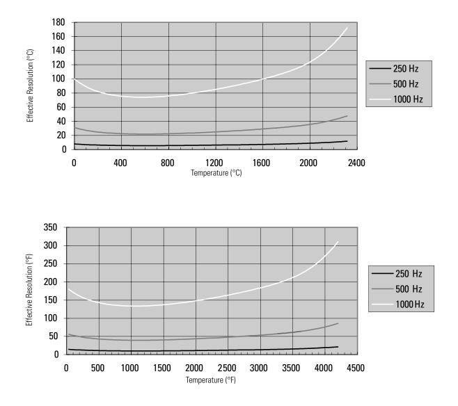
Figure 3.5 Effective Resolution Versus Input Filter Selection for Type C Thermocouples Using 250, 500, and 1k Hz Filters
