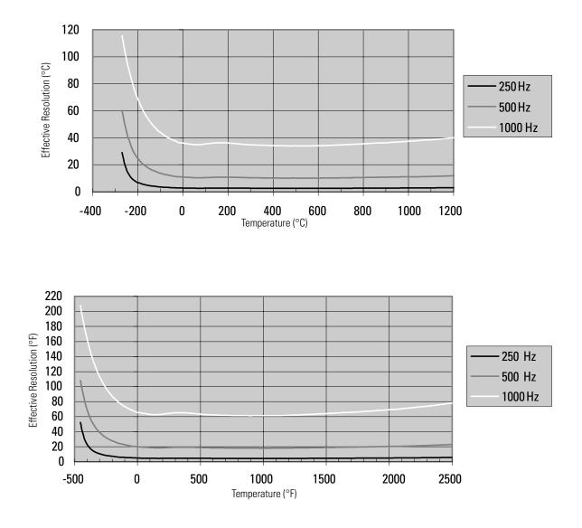
Figure 3.11 Effective Resolution Versus Input Filter Selection for Type K Thermocouples Using 250, 500, and 1k Hz Filters
