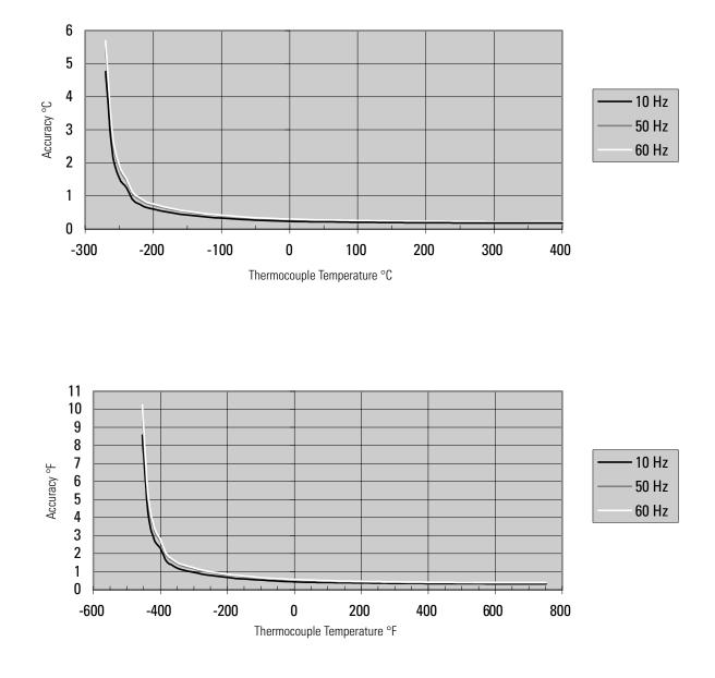
Figure A.17 Module Accuracy at 25°C (77°F) Ambient for Type T Thermocouple Using 10, 50, and 60 Hz Filter
