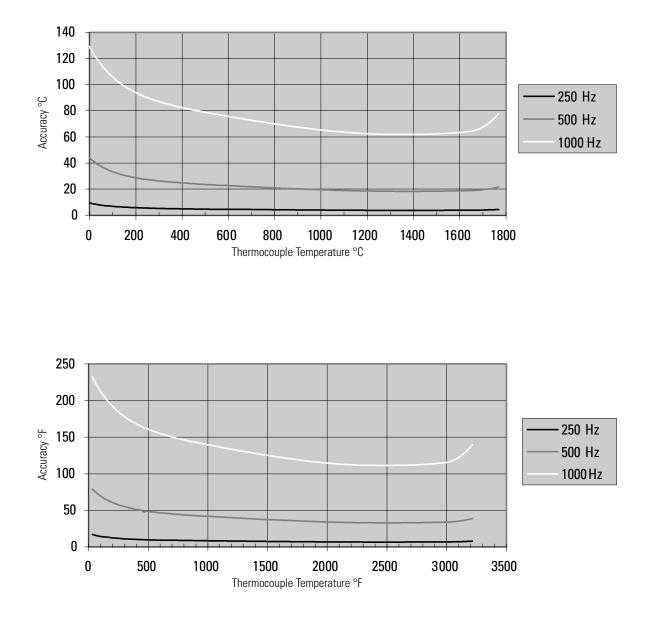
Figure A.14 Module Accuracy at 25°C (77°F) Ambient for Type R Thermocouple Using 250, 500, and 1 kHz Filter
