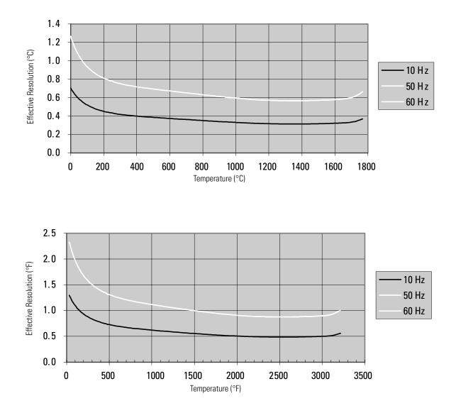
Figure 3.16 Effective Resolution Versus Input Filter Selection for Type S Thermocouples Using 10, 50, and 60 Hz Filters
