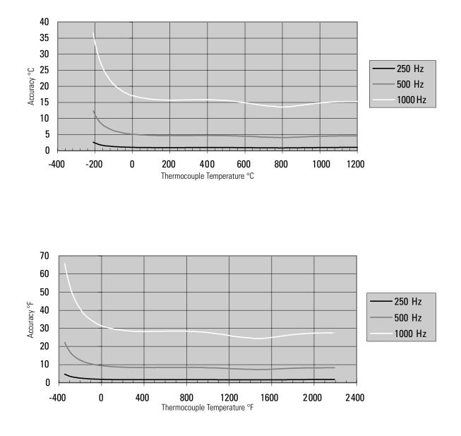
Figure A.8 Module Accuracy at 25°C (77°F) Ambient for Type J Thermocouple Using 250, 500, and 1 kHz Filter
