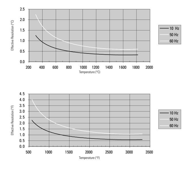
Figure 3.2 Effective Resolution Versus Input Filter Selection for Type B Thermocouples Using 10, 50, and 60 Hz Filters
