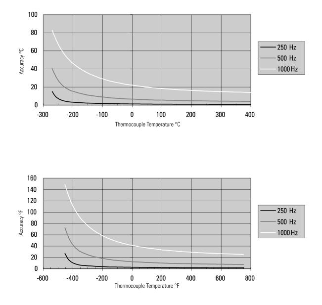
Figure A.18 Module Accuracy at 25°C (77°F) Ambient for Type T Thermocouple Using 250, 500, and 1 kHz Filter
