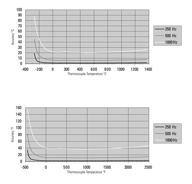
Figure A.10 Module Accuracy at 25°C (77°F) Ambient for Type K Thermocouple Using 250, 500, and 1 kHz Filter
