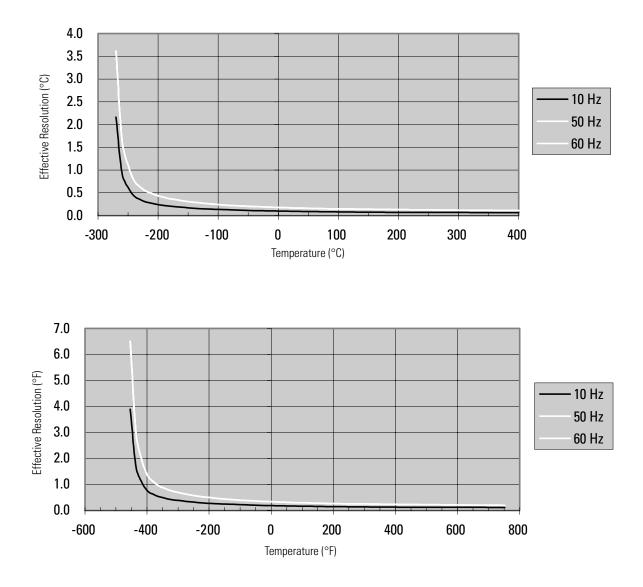
Figure 3.18 Effective Resolution Versus Input Filter Selection for Type T Thermocouples Using 10, 50, and 60 Hz Filters
