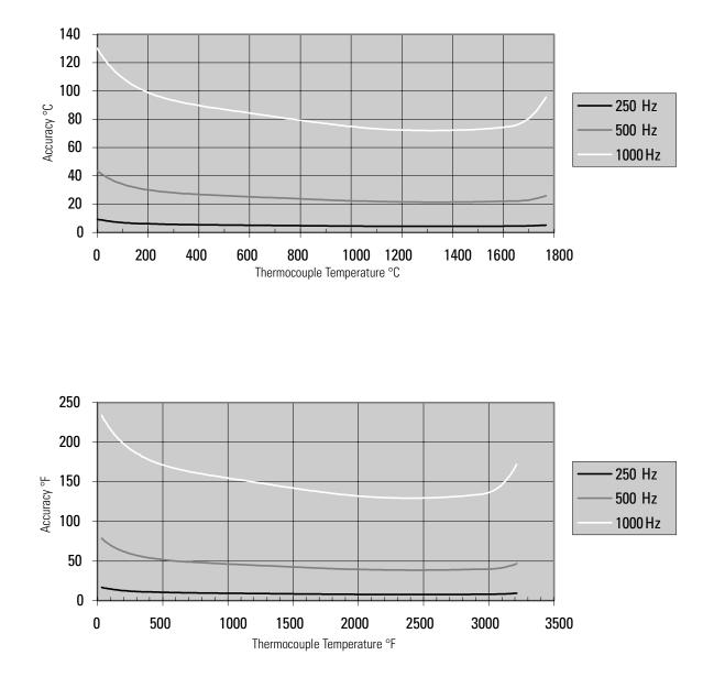
Figure A.16 Module Accuracy at 25°C (77°F) Ambient for Type S Thermocouple Using 250, 500, and 1 kHz Filter
