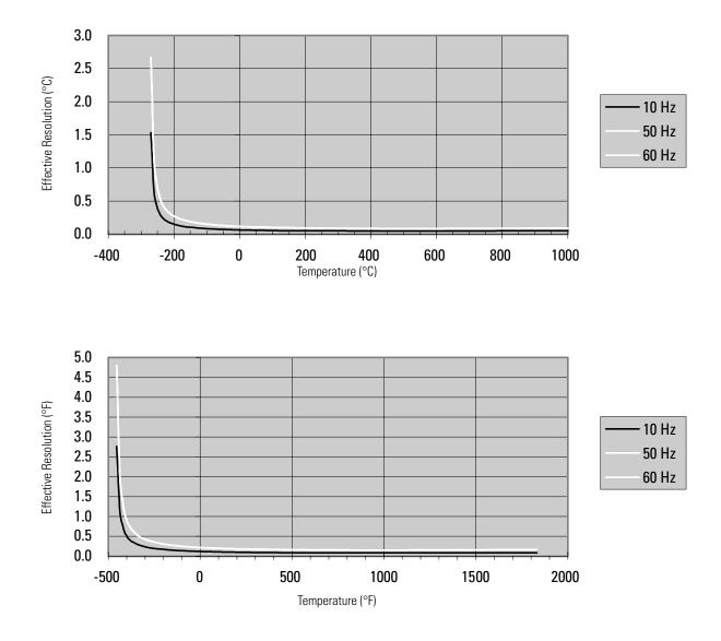
Figure 3.6 Effective Resolution Versus Input Filter Selection for Type E Thermocouples Using 10, 50, and 60 Hz Filters
