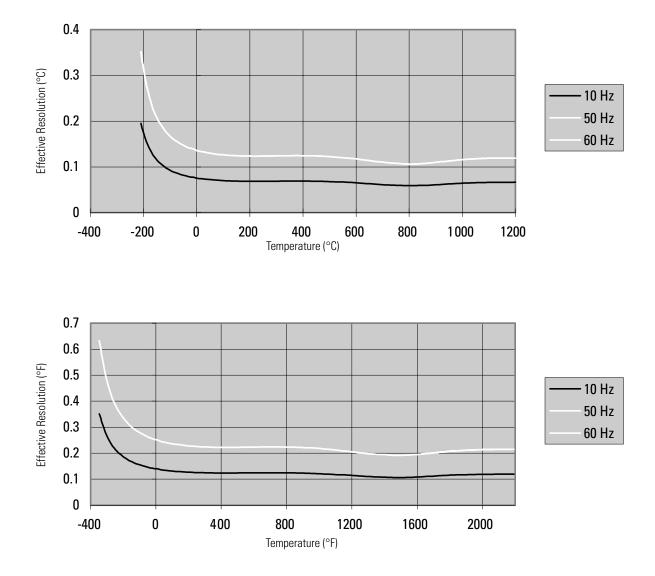
Figure 3.8 Effective Resolution Versus Input Filter Selection for Type J Thermocouples Using 10, 50, and 60 Hz Filters
