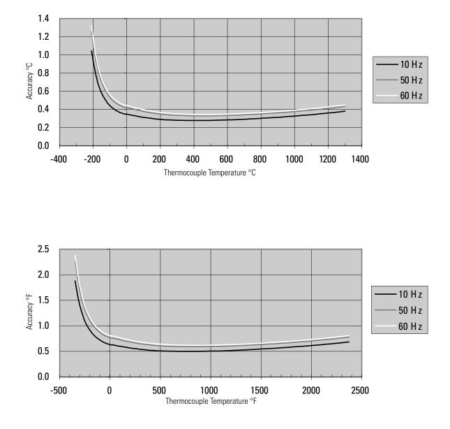
Figure A.11 Module Accuracy at 25°C (77°F) Ambient for Type N Thermocouple Using 10, 50, and 60 Hz Filter
