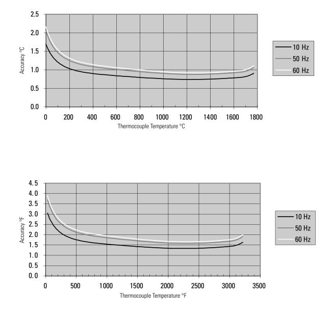
Figure A.13 Module Accuracy at 25°C (77°F) Ambient for Type R Thermocouple Using 10, 50, and 60 Hz Filter
