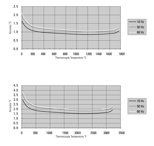
Figure A.15 Module Accuracy at 25°C (77°F) Ambient for Type S Thermocouple Using 10, 50, and 60 Hz Filter
