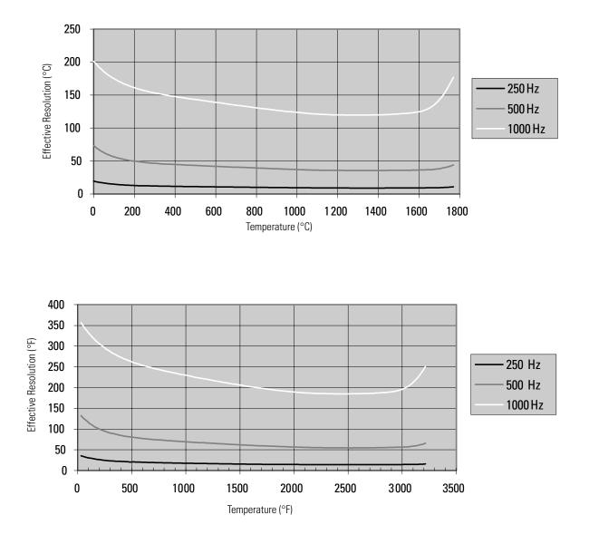
Figure 3.17 Effective Resolution Versus Input Filter Selection for Type S Thermocouples Using 250, 500, and 1k Hz Filters
