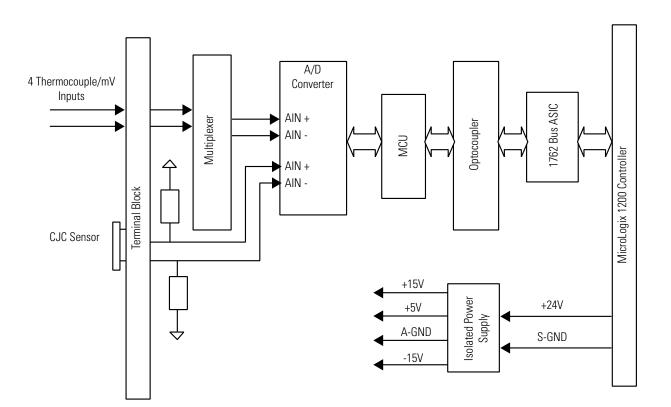
Each channel can receive input signals from a thermocouple or millivolt analog input device, depending upon how you configured the channel.
