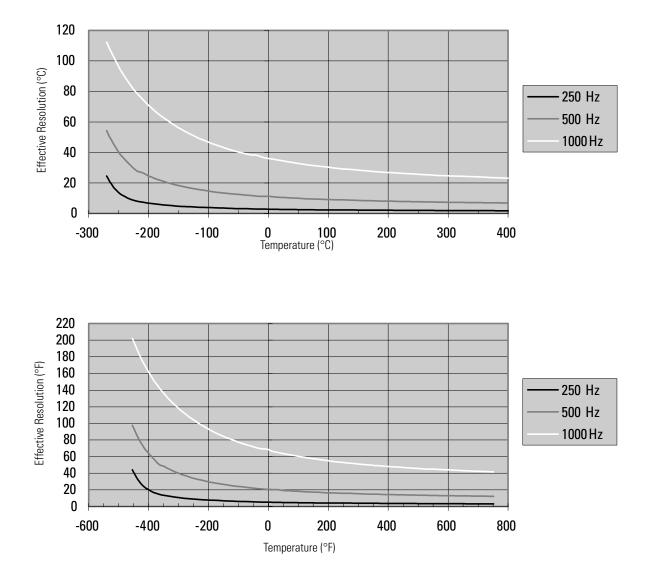
Figure 3.19 Effective Resolution Versus Input Filter Selection for Type T Thermocouples Using 250, 500, and 1k Hz Filters
