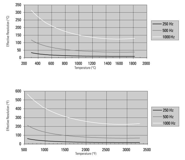
Figure 3.3 Effective Resolution Versus Input Filter Selection for Type B Thermocouples Using 250, 500, and 1k Hz Filters
