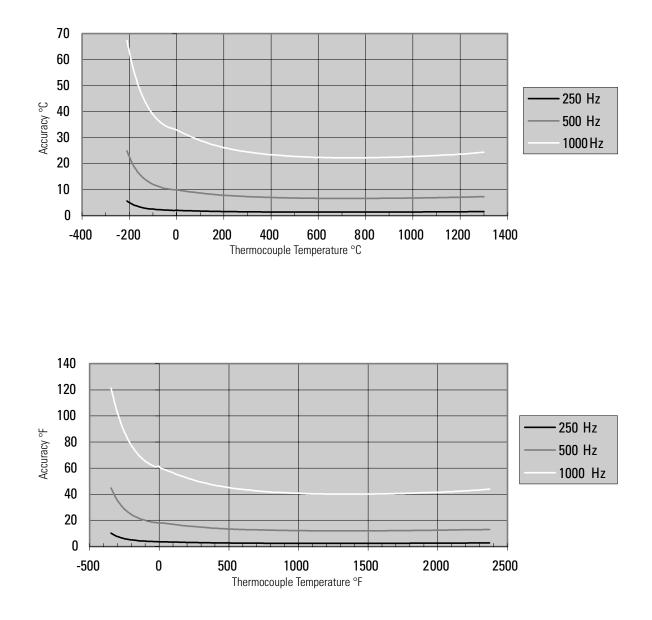
Figure A.12 Module Accuracy at 25°C (77°F) Ambient for Type N Thermocouple Using 250, 500, and 1 kHz Filter
