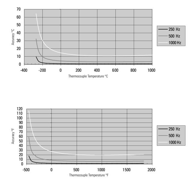
Figure A.6 Module Accuracy at 25°C (77°F) Ambient for Type E Thermocouple Using 250, 500, and 1 kHz Filter
