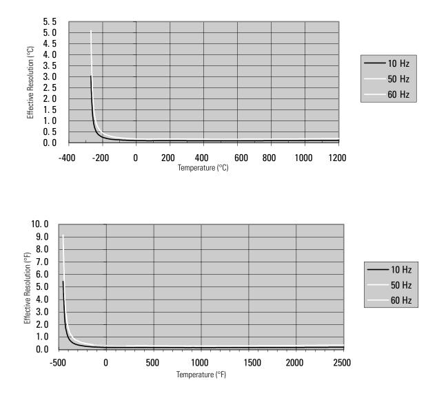
Figure 3.10 Effective Resolution Versus Input Filter Selection for Type K Thermocouples Using 10, 50, and 60 Hz Filters
