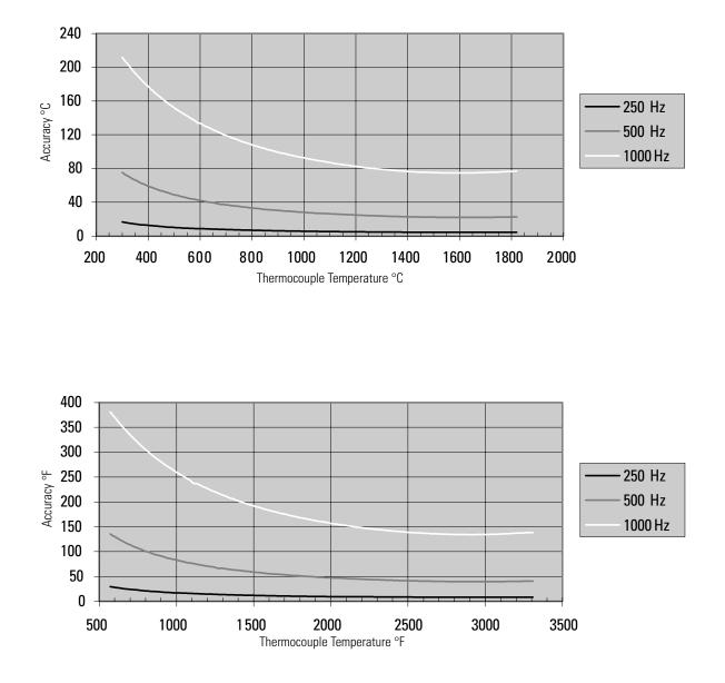
Figure A.2 Module Accuracy at 25°C (77°F) Ambient for Type B Thermocouple Using 250, 500, and 1 kHz Filter
