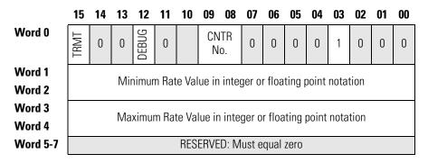
Figure 4.7 Min./Max. Rate Value Block
