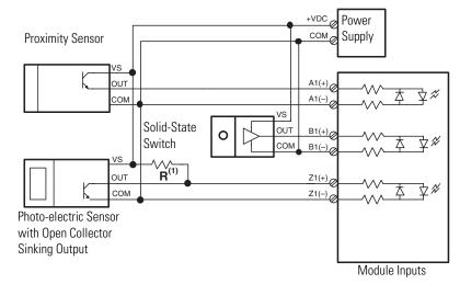
(1) Calculate the value of the pull-up resistor (R), as shown below:
