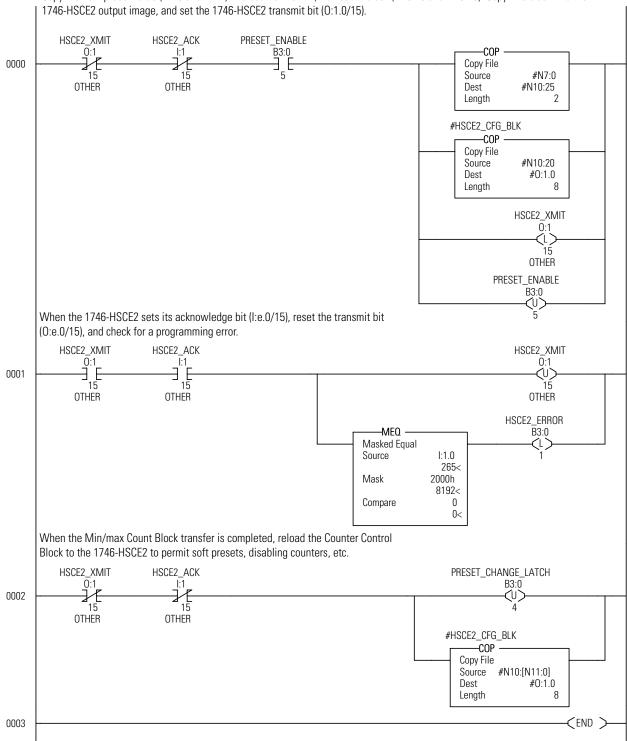
Copy the new preset value (N7:0 and N7:1) into counter 1's min/max count block (N10:25 and N10:26). Copy this block into the
