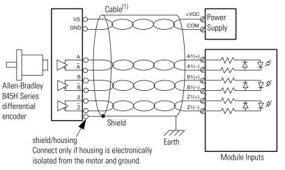
Refer to your encoder manual for proper cable type. The type of cable used should be twisted pair, individually shielded cable with a maximum length of 300m (1000 ft.).
