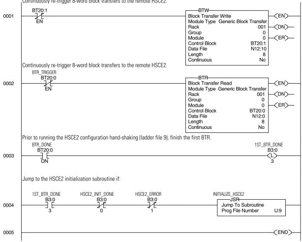
Continuously re-trigger 8-word block transfers to the remote HSCE2.
