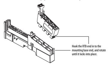
2. Rotate the terminal block into the mounting base until it locks itself in place.
