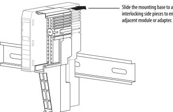
Slide the mounting base to allow the interlocking side pieces to engage the **3.** Press firmly to seat the mounting base on the DIN rail. The mounting base snaps into place.
