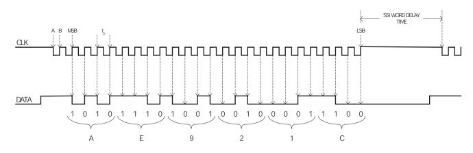
The CLK and DATA signals are representative of what you could actually see on an oscilloscope when the module is attached to a SSI sensor in a live system. The SSI module must be configured for a SSI Word length of 24, as well as the proper Data Rate and SSI Word Delay time stated in the SSI sensor specifications.
