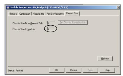
Notice the chassis size in the module is modified to 3.
