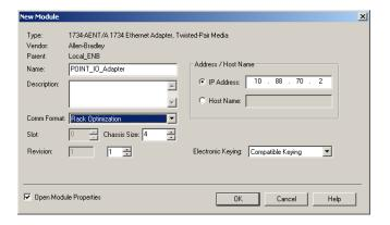
**4.** Enter values for Name, IP Address, Comm Format, Chassis Size, Electronic Keying, and Revision, noting we used the following values.
