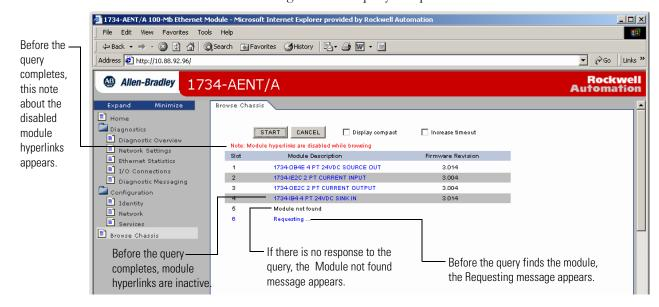
After completion of a query, here is how a typical Browse Chassis page looks with the module hyperlinks active and the Display compact check box unchecked.
