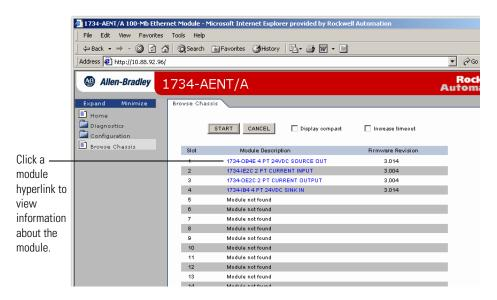
Here is how a typical Browse Chassis page looks with the Display compact check box checked.
