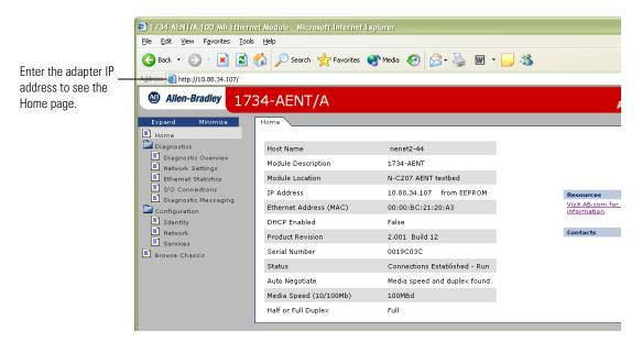
**2.** From the Home page, click Expand to expand options, as in the figure, or Minimize to see Diagnostics, Configuration, and Browse Chassis options without the expansion.
