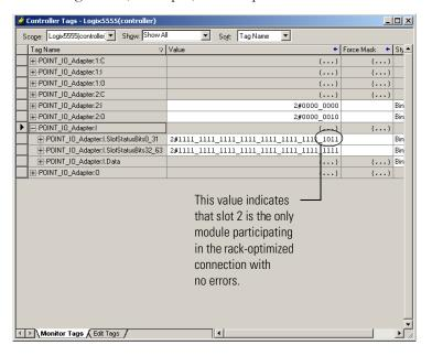
Use the controller tags in your ladder program to read input data or write output data.
