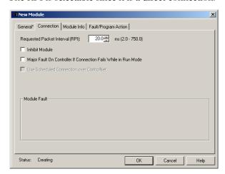
**6.** Enter 50 for requested packet interval (RPI) to set how often you exchange data with the 1734-AENT adapter.
