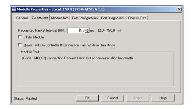
If you encounter this condition, the only action you can take is to alter the existing connections to reduce the amount of microprocessor bandwidth consumed. The most likely fixes for this condition include the following.
