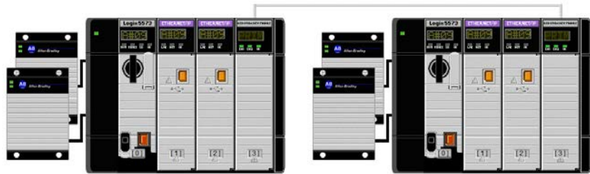
Figure 3 - Redundancy System Configuration Example
