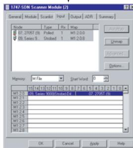
Select the Output tab and click AutoMap to automatically map output devices.
