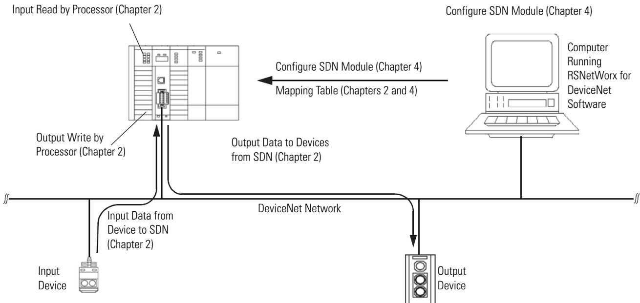
The 1747-SDN interface module can also be used to bridge a DeviceNet network with another network.
