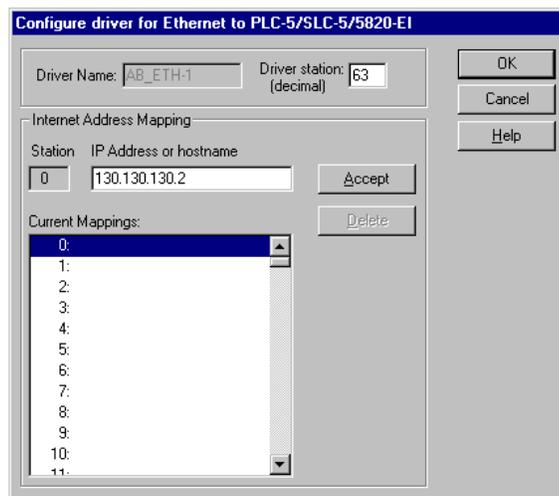
5. Enter the IP address of the SLC 5/05 processor in the IP address or hostname field (130.130.130.2 in this example).
