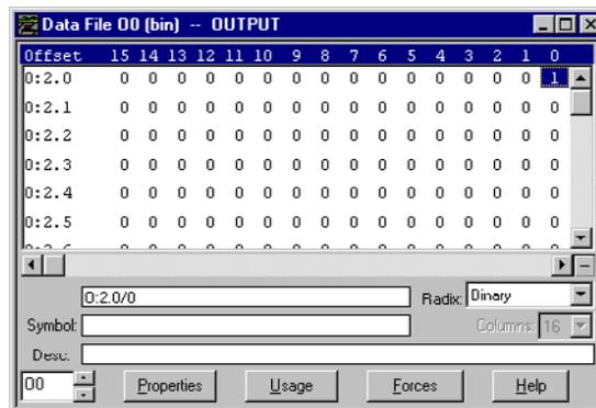
6. Set bit 0 in the command register to 1, as shown above.
