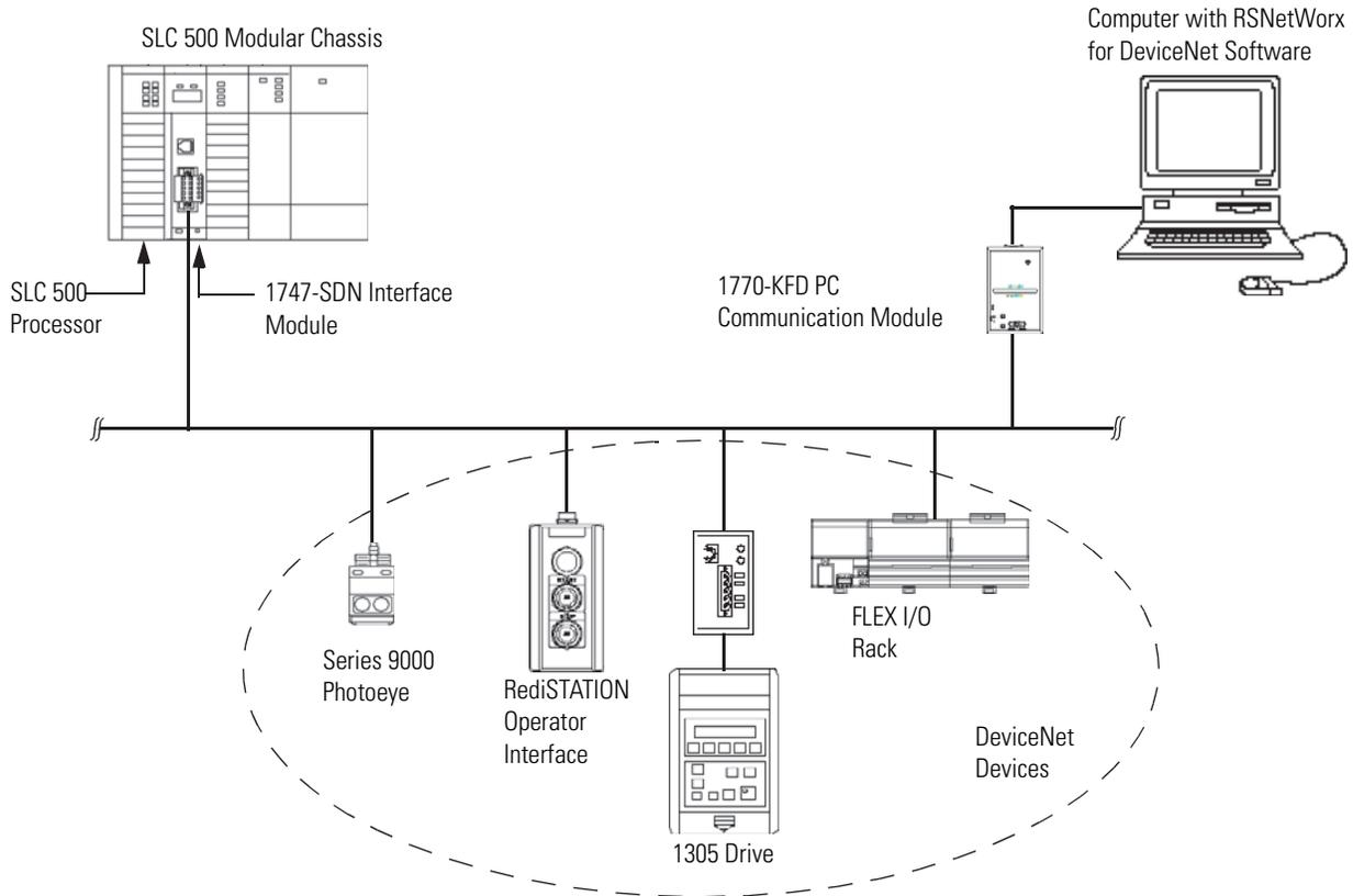
The 1747-SDN module communicates with DeviceNet devices over the network to:
