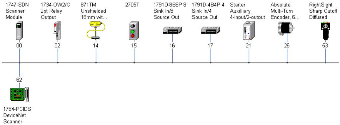
The node addresses can be commissioned via hardware switches on the device or through other DeviceNet configurators such as the 193-DNCT DeviceNet Configuration terminal.
