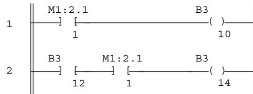
XIC instructions in rungs 1 and 2 are addressed to the M1 data file. Each of these instructions adds approximately 1 ms to the scan time (SLC 5/02, series B processor).
