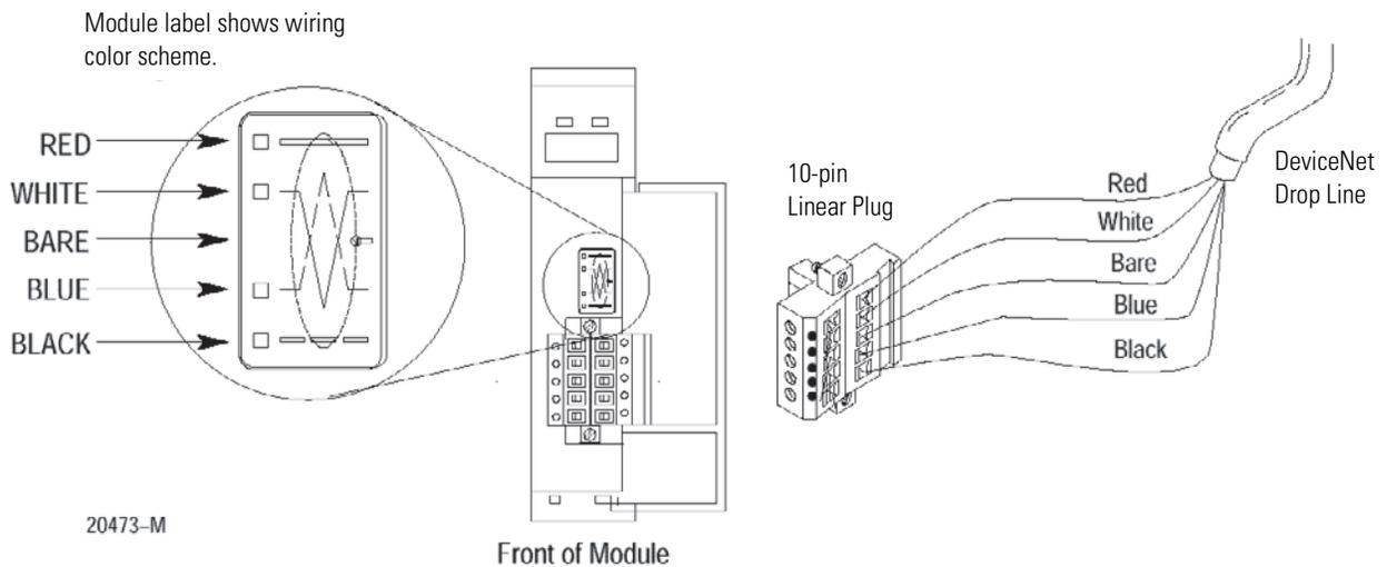
3. Locate the DeviceNet port connector on the front of the module, and insert the 10-pin linear plug into the connector.
