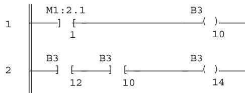
These rungs provide equivalent operation to those of the previous diagram by substituting XIC instruction B3/10 for XIC instruction M1:2.1/1 in rung 2. Scan time is reduced by approximately 1 ms (SLC 5/02 series B processor).
