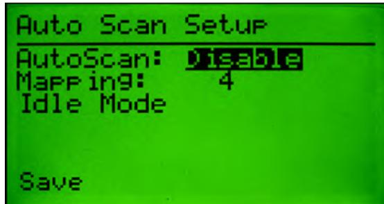
7. Press the B/SEL key to scroll down to Mapping.
