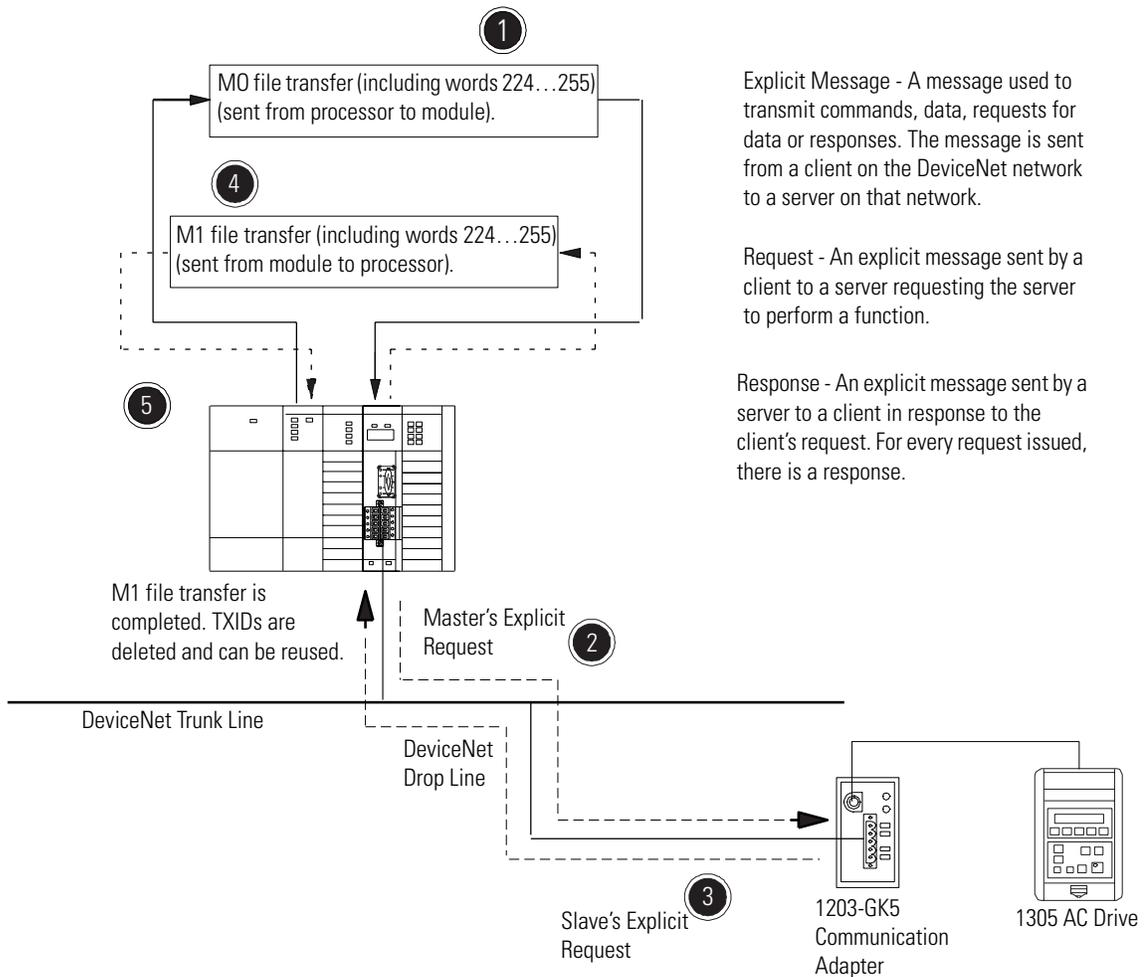
Explicit Message - A message used to transmit commands, data, requests for data or responses. The message is sent from a client on the DeviceNet network to a server on that network.
