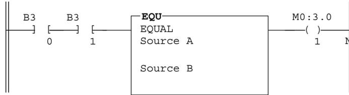
This rung does not show its true rung state because the EQU instruction is always shown as true and the M0 instruction is always shown as false.
