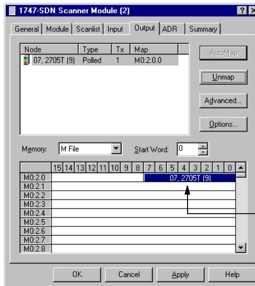
After mapping, the RediSTATION output address appears here.
