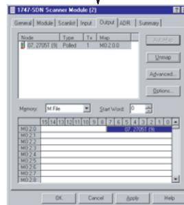
Double-click the device in the scanlist to edit a device's I/O parameters.
