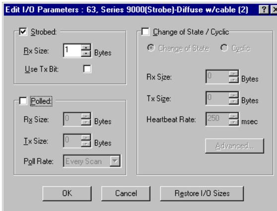
The I/O parameters define the configuration for the device in terms of how much and what data the device exchanges with the 1747-SDN module. By default, the photoeye will send 1 byte when it receives the strobe request.
