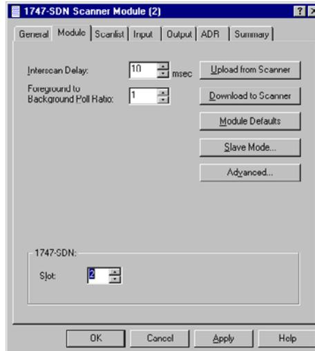
4. Verify the 1747-SDN module slot number is correct for your system.
