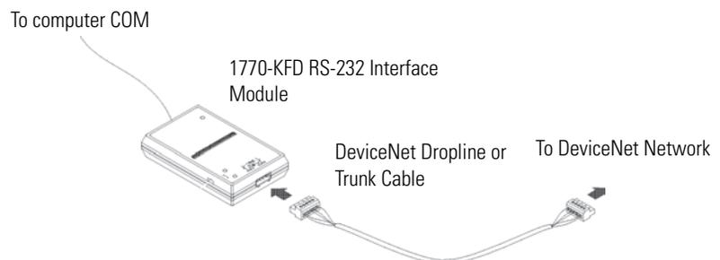
For detailed directions on how to install the 1770-KFD module, see the DeviceNet RS-232 Interface Module Installation Instructions, publication 1770-5.6.
