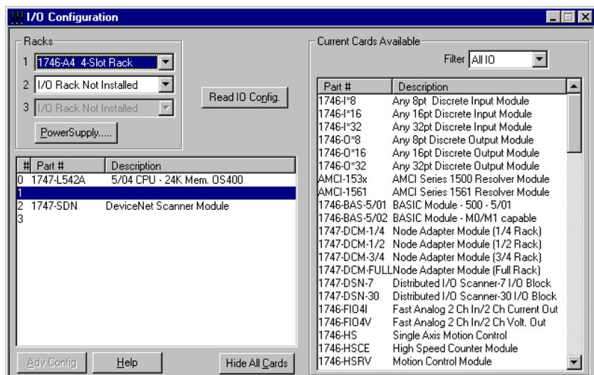
3. Click Read I/O Config to upload the I/O configuration from the processor.
