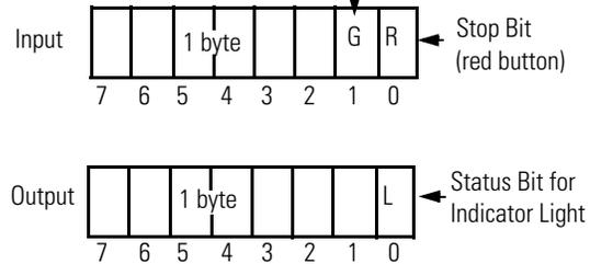
One output bit for the RediSTATION operator interface's indicator light (on/off) will be mapped.
