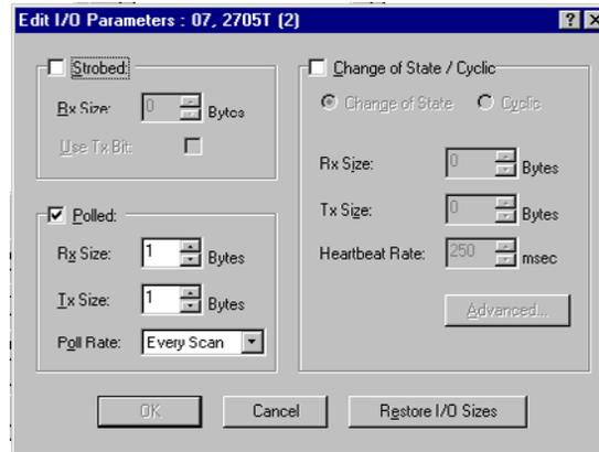
2. Verify that the Polled box is checked and that the Rx Size and Tx Size are each 1 byte.
