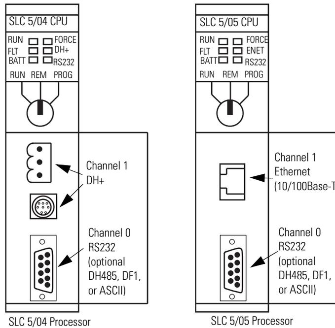
Make sure system power is off; then insert the processor into slot 0 of the 1746 I/O chassis.
