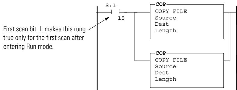
First scan bit. It makes this rung true only for the first scan after entering Run mode.
