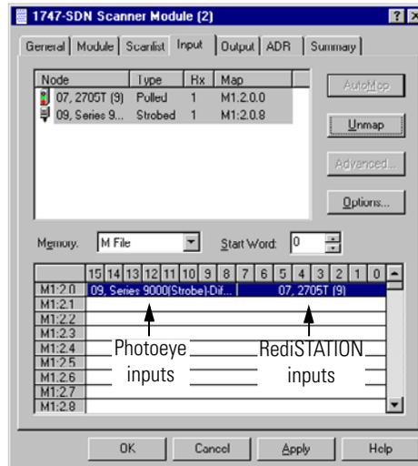
In this example, the inputs from the RediSTATION operator interface appear in the M1 file for the device in slot 2 as word 0, bits 0...7.
