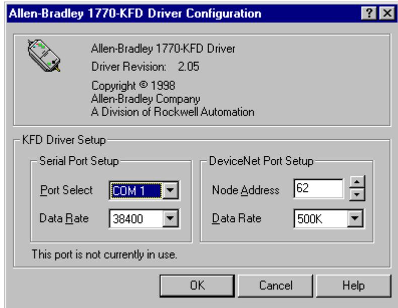
5. Configure the driver by using the example above as a guide and click on OK.
