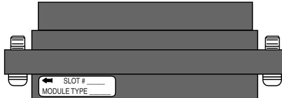
To remove the terminal block, loosen the upper and lower retaining screws. The terminal block will back away from the module as you remove the screws. When replacing the terminal block, torque the retaining screws to 0.46 Nm (4.1 lb-in).
