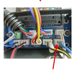
$\ensuremath{^{*}}$  Remove the adapter box and connect the auto-leveler port here.
