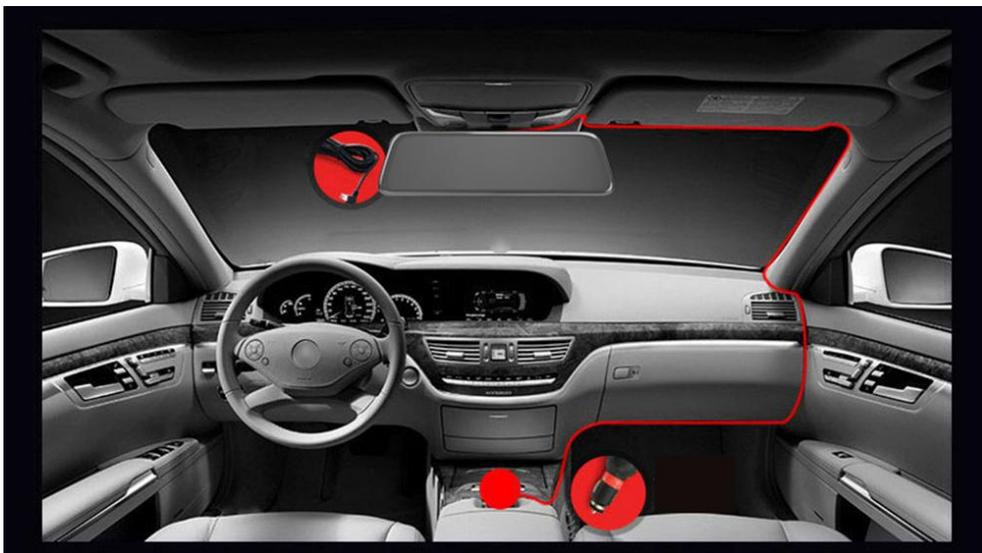
1. Please pull out the front lens before installation to avoid length limitation and cannot be installed;
