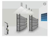
With movement and insufficient ambient lux level, the light is triggered on 100% by the detector.
