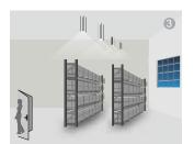
If there is no more movement, the light dims to stand-by dimming level after hold-time.
