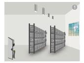
The light keeps off during daytime even when movement is detected. (Ambient lux level is above preset daylight threshold)
