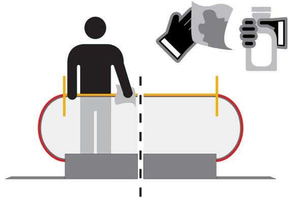
3. Advance escalator to expose next section of handrail, repeat process until complete.
