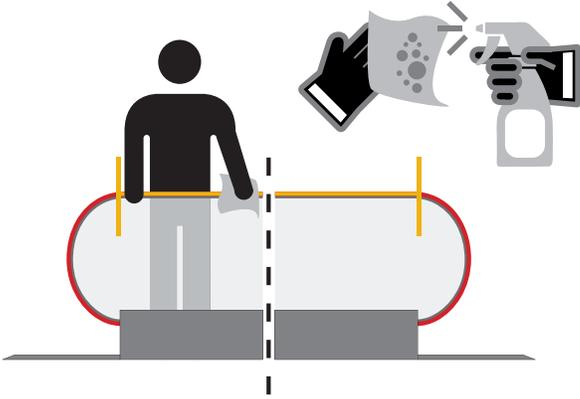
3. Advance escalator to expose next section of handrail, repeat process until complete.
